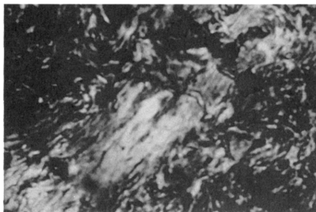
Figure 17. Texture of the nematic phase of copolyester C2 at T = 380 °C. Crossed polarizers.
